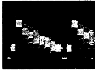
3 Pin 38 of IC301 (SECAM color bar output : 2.0Vp-p)
